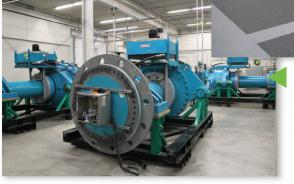
In 2020, NextEra Energy donated gearboxes and hubs to transform our indoor Wind Turbine Technology lab. The 30-ton gearboxes rest on stands fabricated by our own Welding and Manufacturing department. This lab gives students the chance to troubleshoot and repair equipment on the ground, simulating what they would find inside a wind tower 300 feet in the air.
